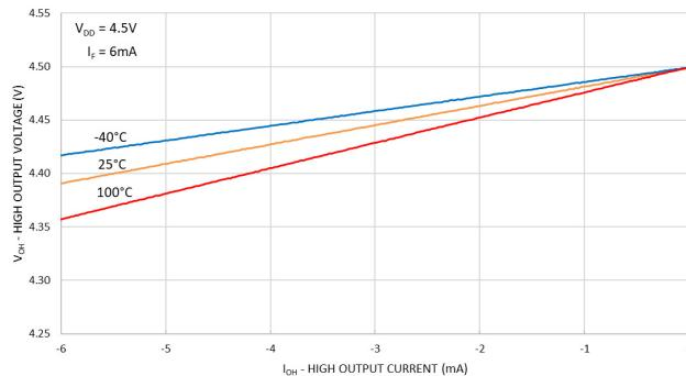
**Figure 9.  $V_{O\text{H}}$  vs.  $I_{O\text{H}}$  Across Temperatures**
