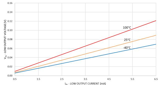
**Figure 10.  $V_{O\text{I}}$  vs.  $I_{O\text{I}}$  Across Temperatures**
