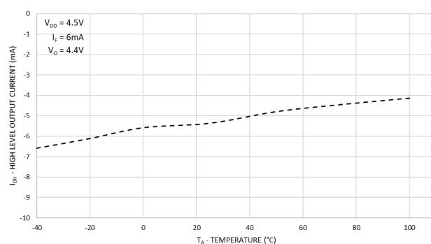
**Figure 2. Typical Logic High Output Current vs. Temperature**
