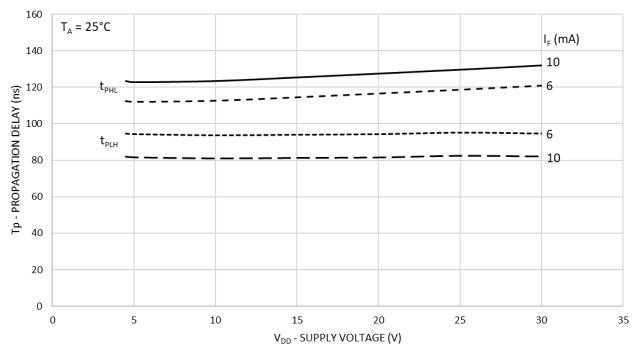
**Figure 8. Typical Propagation Delay vs. Supply Voltage**
