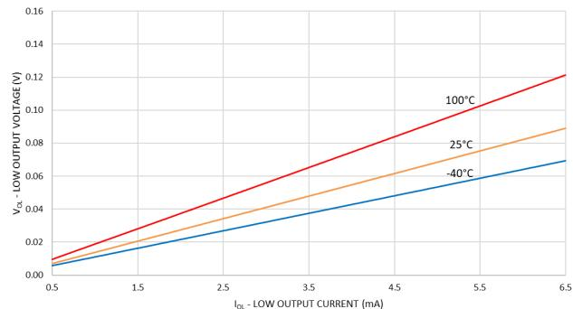
**Figure 10.  $V_{O\text{I}}$  vs.  $I_{O\text{I}}$  Across Temperatures**
