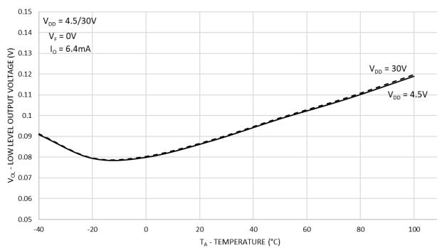
**Figure 1. Typical Logic Low Output Voltage vs. Temperature**
