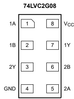
Fig. 5. Pin configuration SOT833-1, SOT1089, SOT1116 and SOT1203
