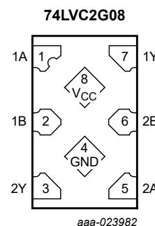
Fig. 7. Pin configuration SOT1233
