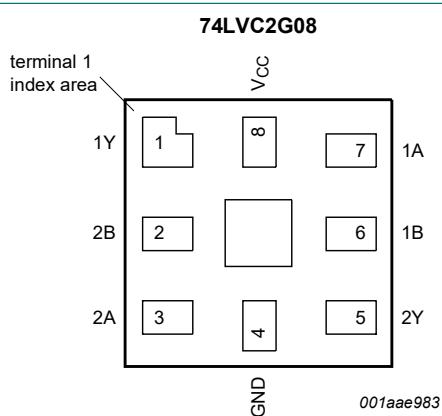
Fig. 6. Pin configuration SOT902-2
