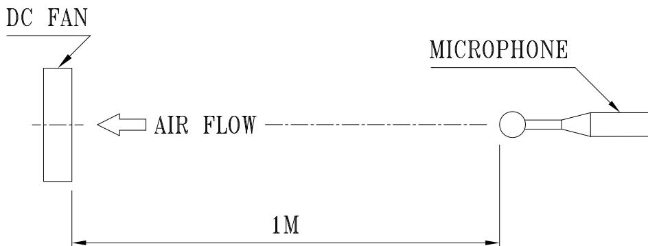
NOISE IS MEASURED AT RATED VOLTAGE IN FREE AIR IN ANECHOIC
