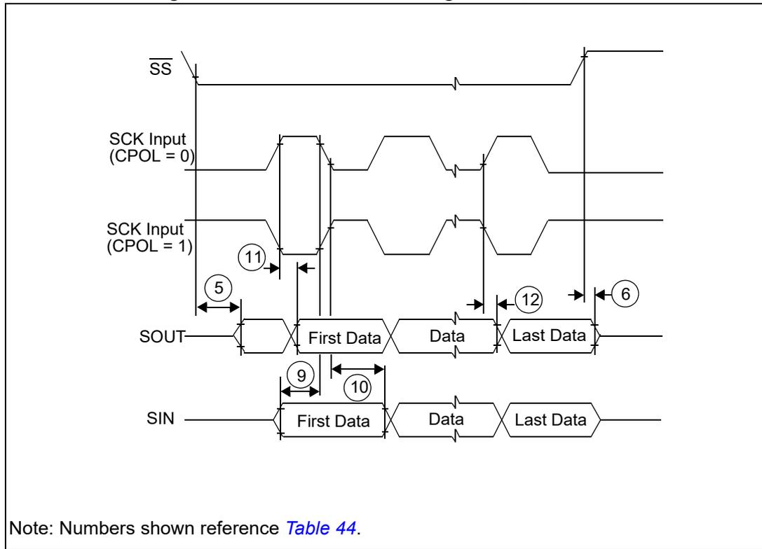
Figure 20. DSPI modified transfer format timing – master, CPHA = 0
