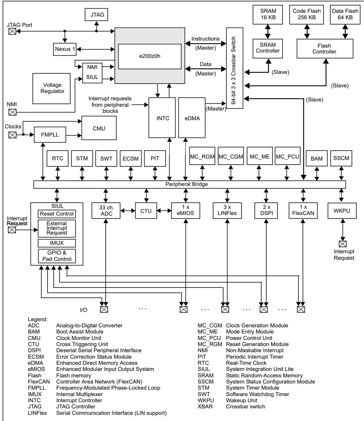
Table 3 summarizes the functions of all the blocks present in the SPC560D30x and SPC560D40x series of microcontrollers. Note that the presence and number of blocks varies by device and package.
