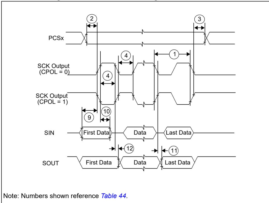
Figure 17. DSPI classic SPI timing – master, CPHA = 1
