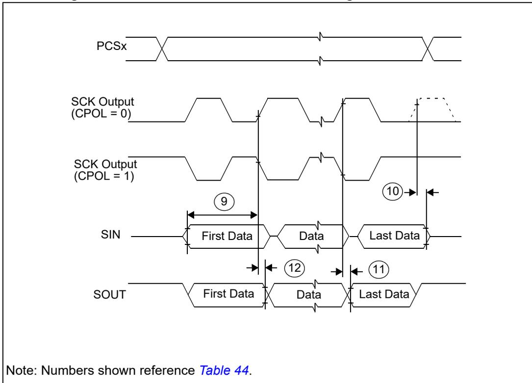
Figure 22. DSPI modified transfer format timing – slave, CPHA = 0
