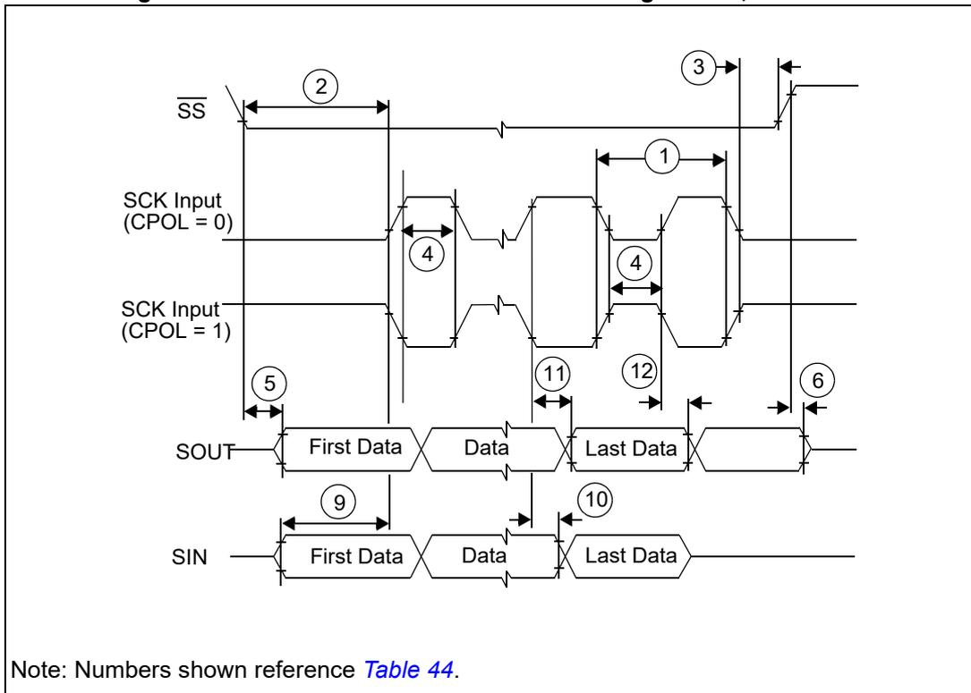
Figure 23. DSPI modified transfer format timing – slave, CPHA = 1
