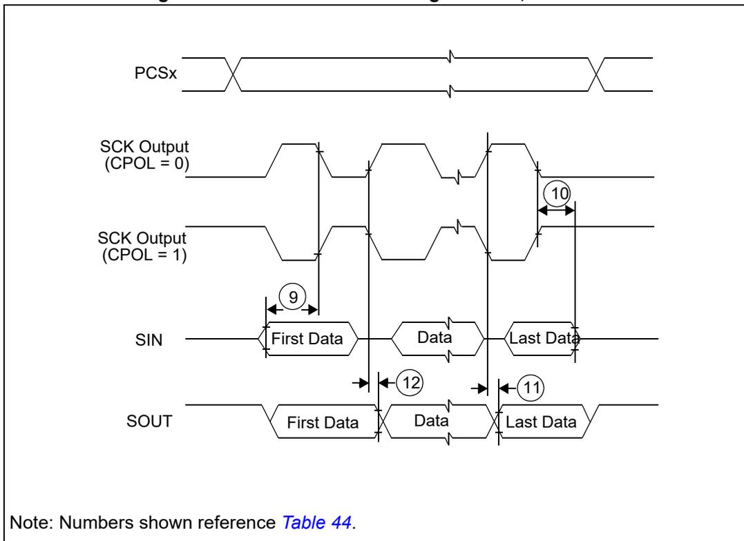
Figure 18. DSPI classic SPI timing – slave, CPHA = 0
