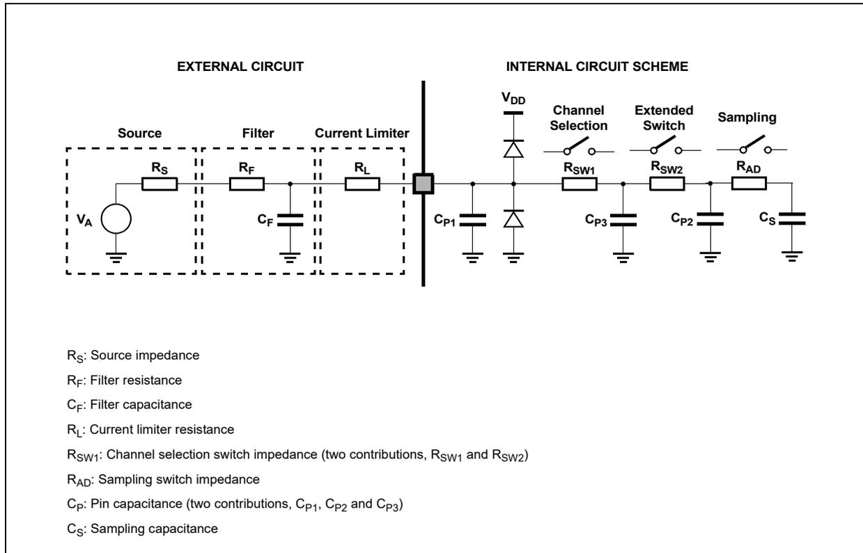
A second aspect involving the capacitance network shall be considered. Assuming the three capacitances  $C_F$ ,  $C_{P1}$  and  $C_{P2}$  are initially charged at the source voltage  $V_A$  (refer to the equivalent circuit in [Figure 13](#)): A charge sharing phenomenon is installed when the sampling phase is started (A/D switch close).
