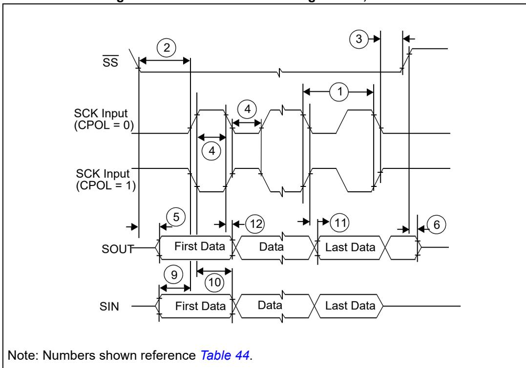
Figure 19. DSPI classic SPI timing – slave, CPHA = 1
