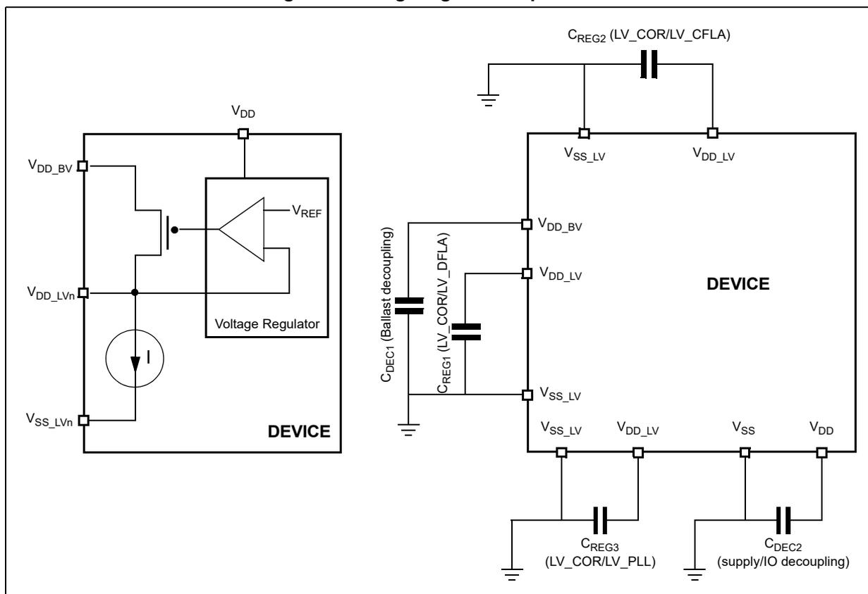
The internal voltage regulator requires external capacitance ( $C_{REGn}$ ) to be connected to the device in order to provide a stable low voltage digital supply to the device. Capacitances should be placed on the board as near as possible to the associated pins. Care should also be taken to limit the serial inductance of the board to less than 5 nH.
