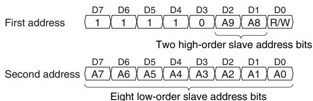
Figure 13.4.4.1 10-bit Address Configuration
