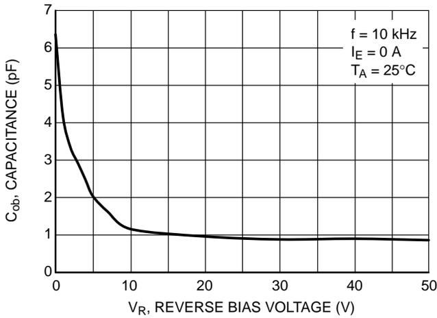
Figure 9. Output Capacitance
