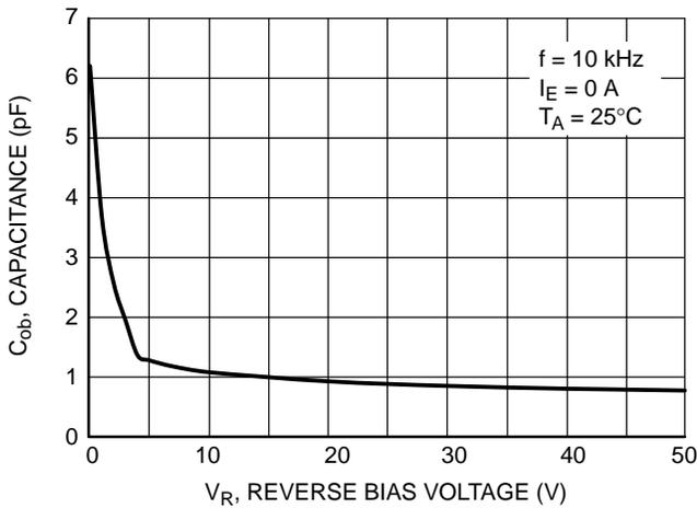
Figure 4. Output Capacitance
