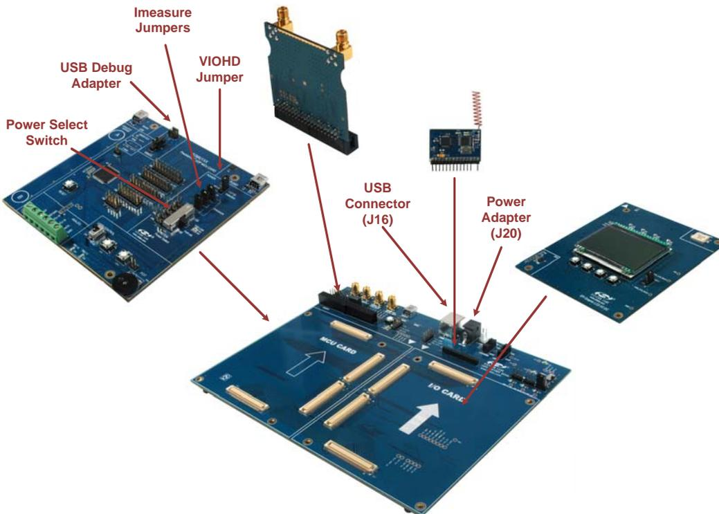
Figure 3. Hardware Setup using the Unified Development Platform
