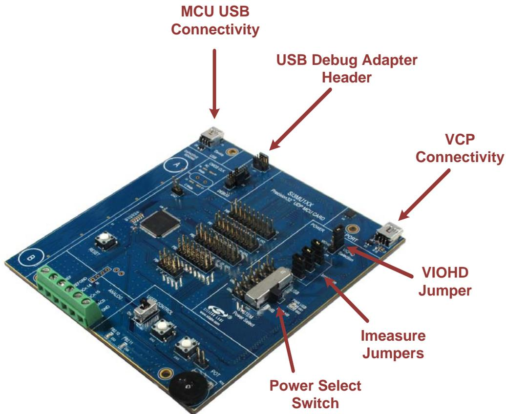
Figure 2. Hardware Setup using the MCU Card Alone
