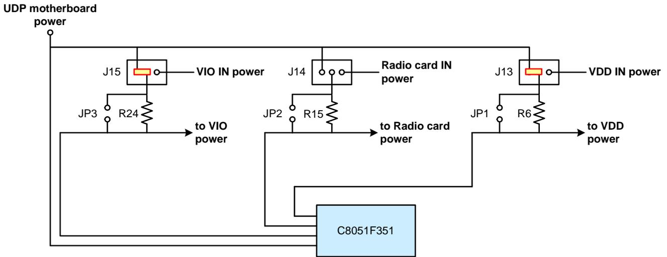
Figure 7. Power Measurement Diagram with Shorting Blocks
