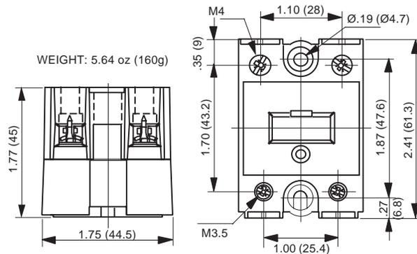
Figure 1 – XV relay; dimensions in inches (mm)
