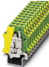
Ground terminal block with screw connection, cross section: 0.5 - 10 mm 2 , AWG: 20 - 6, width: 10.2 mm, color: green-yellow
