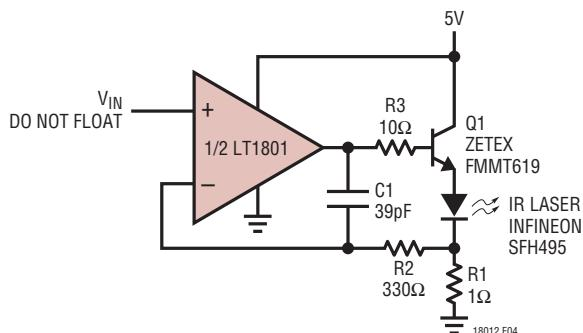
Figure 4. Single Supply 1A Laser Driver Amplifier
