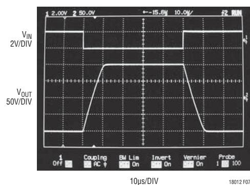
Figure 7. Large-Signal Time Domain Response of the Amplifier
