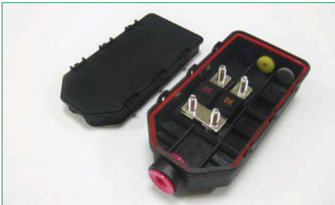
This splash-water-proof fuse holder with cover can be flexible enough to be used with 2 or 3 MIDI® fuses. A Snap-on fixes the sheet metals in the holder. The holder includes M5 threaded bolts and cover seal. Busbar and cable seals are optional. Fuse not included.
