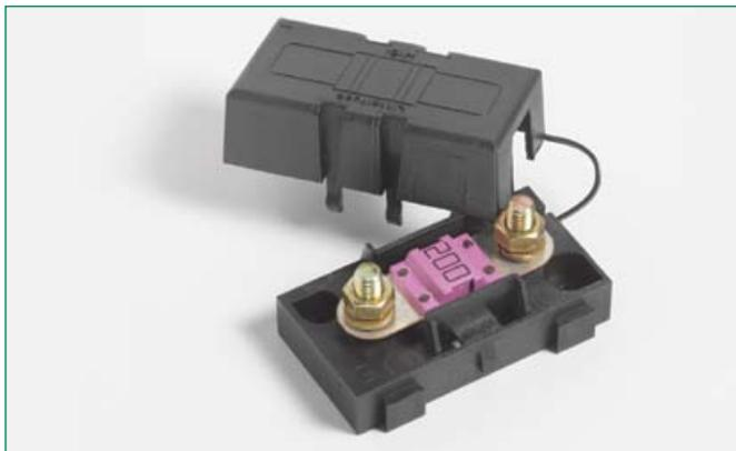
Use with BF1 /MIDI® fuses up to 200A. Includes protective cover. Features interconnecting pins on side of fuse block for secure multiple block configurations. Includes M5 threaded studs and hex nuts with lock washers. Fuse not included.
