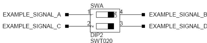
Figure 2-3. Example of Mechanical Switch Equivalent to [Figure 2-2](#)
