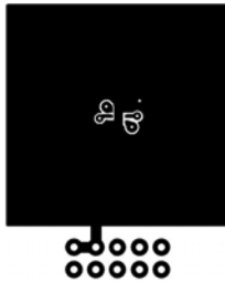
c. 69 °C/W when mounted on a 1 in 2 pad of 2 oz copper
