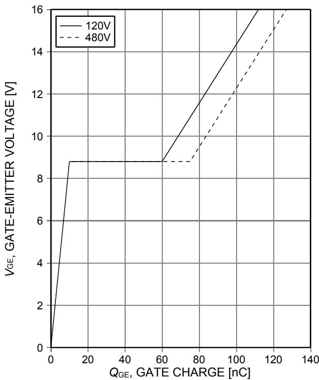
Figure 17. Typical gate charge
