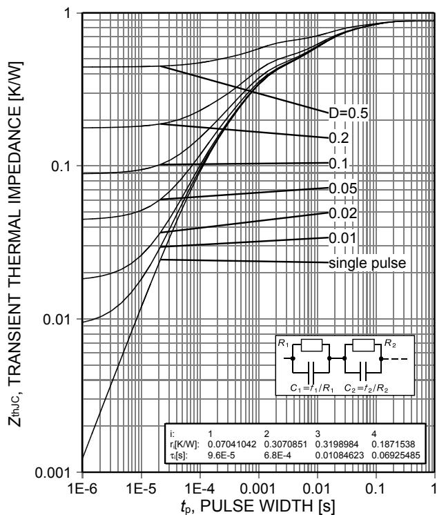
Figure 21. IGBT transient thermal impedance
