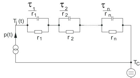
Figure D. Thermal equivalent circuit
