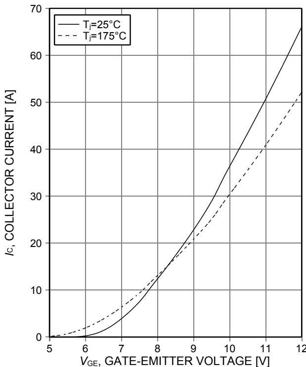
Figure 7. **Typical transfer characteristic**
