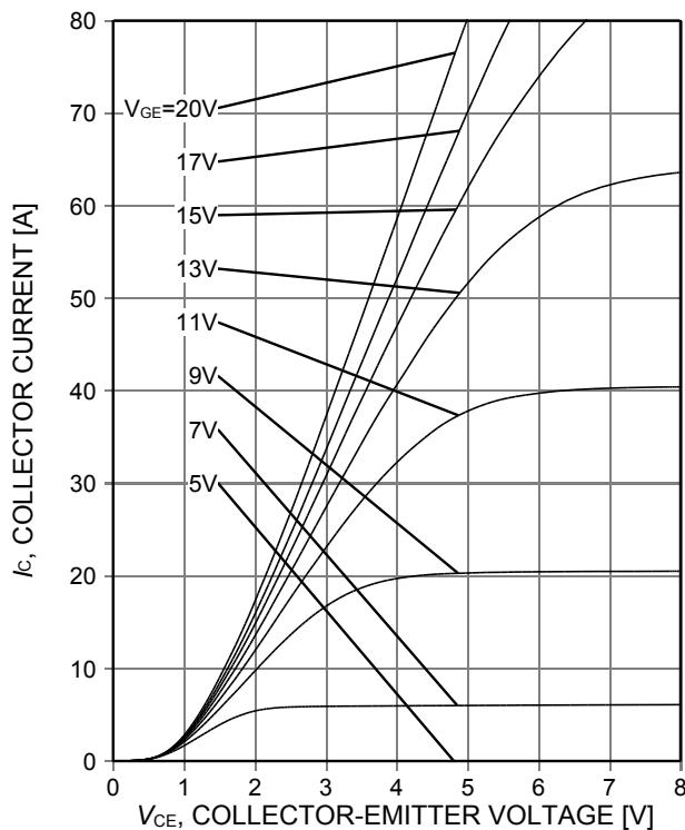
Figure 6. **Typical output characteristic**
