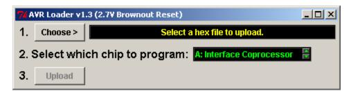
In step 1, click the "Choose" button to bring up a file dialog. Locate the desired AVR .hex file, and click "Open". In step 2, select which coprocessor to load: "A", "B", or both. In step 3, just click the button, and Stampw.exe will be invoked. Once the AVR loader program is uploaded to the BASIC Stamp, a debug window will pop up showing the AVR programming progress. If everything goes okay, the AVR chip(s) will be programmed with the new code.
