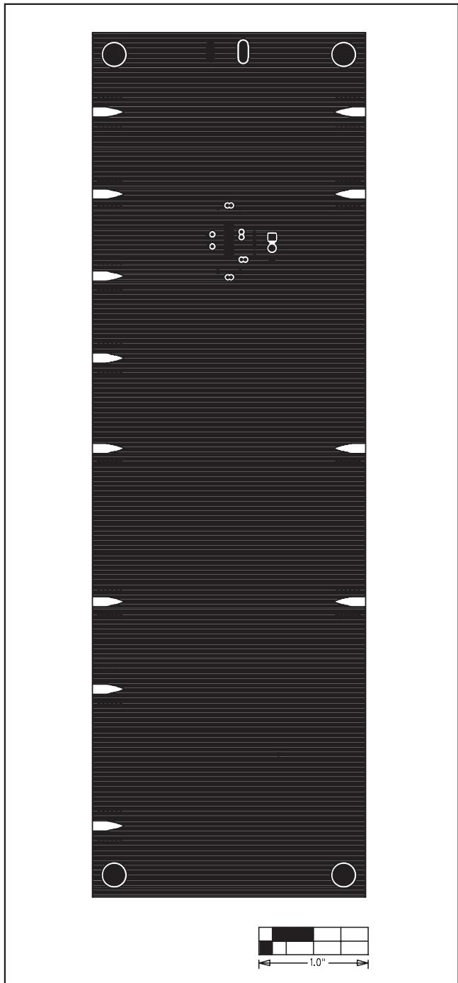
Figure 4. MAX4889B EV Kit PCB Layout—Inner Layer 2
