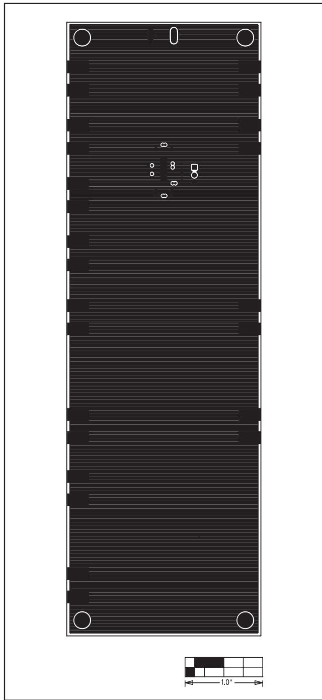
Figure 6. MAX4889B EV Kit PCB Layout—Solder Side
