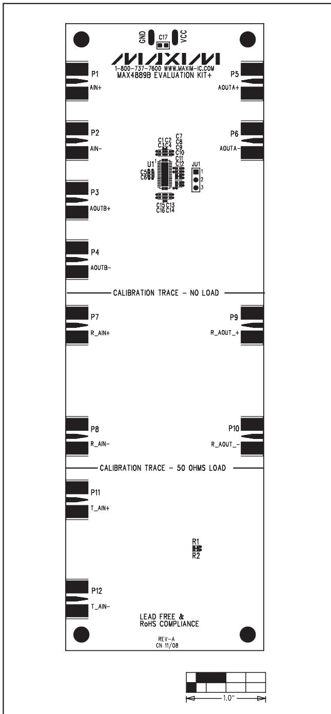
Figure 2. MAX4889B EV Kit Component Placement Guide—Component Side
