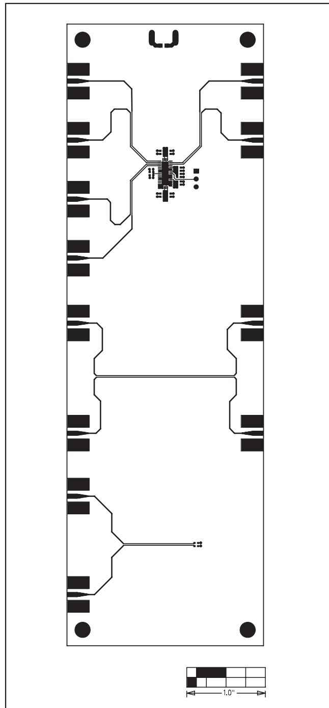
Figure 3. MAX4889B EV Kit PCB Layout—Component Side
