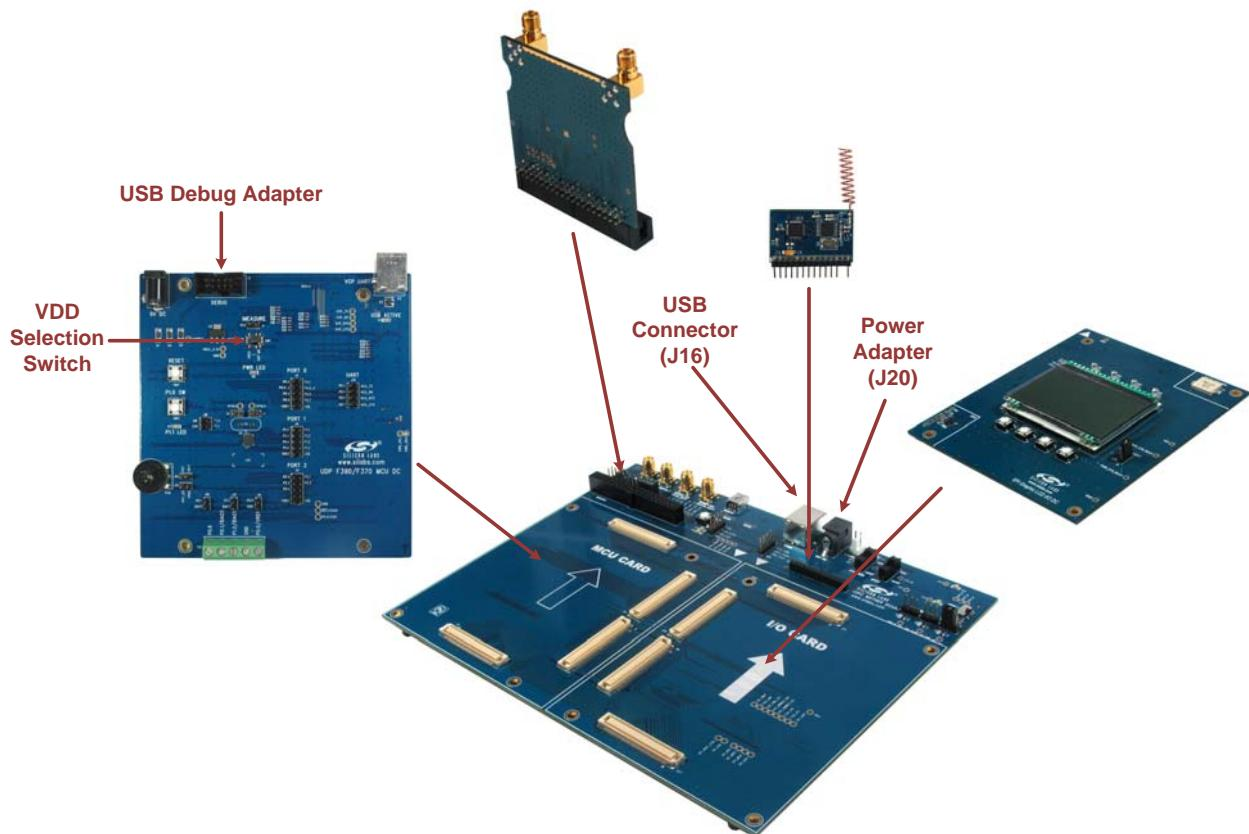
**Figure 3. Hardware Setup using the Unified Development Platform**
