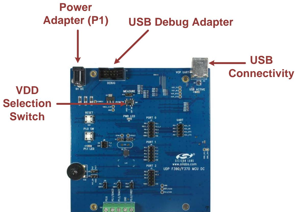
Figure 2. Hardware Setup using the MCU Card Alone
