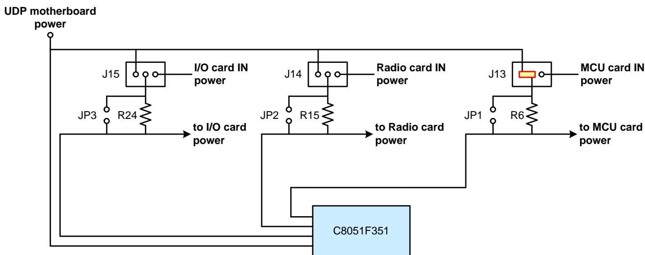
Figure 6. Power Measurement Diagram with Shorting Block
