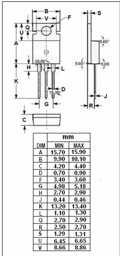
**isc Silicon NPN Power Transistor****MJE2801T****ELECTRICAL CHARACTERISTICS** $T_C=25^\circ\text{C}$  unless otherwise specified
