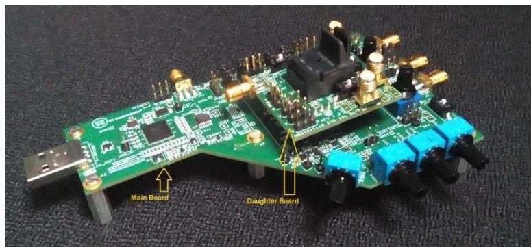
Figure 1. 45° View of Main Board with 16QFN
