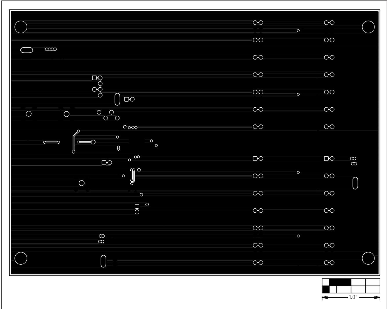
Figure 6. MAX1213/MAX1214/MAX1215 EV Kit PC Board Layout—Solder Side
