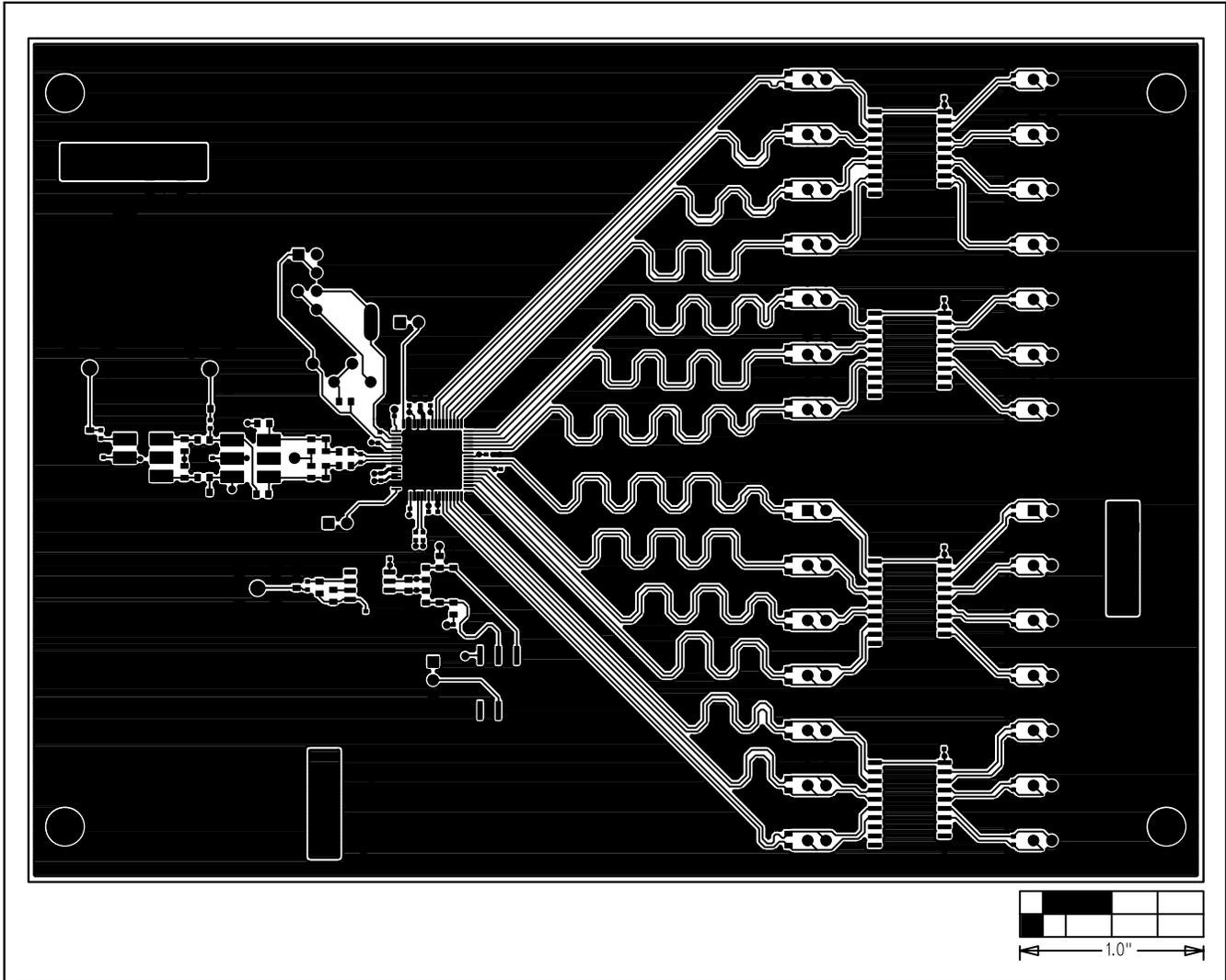
Figure 3. MAX1213/MAX1214/MAX1215 EV Kit PC Board Layout—Component Side
