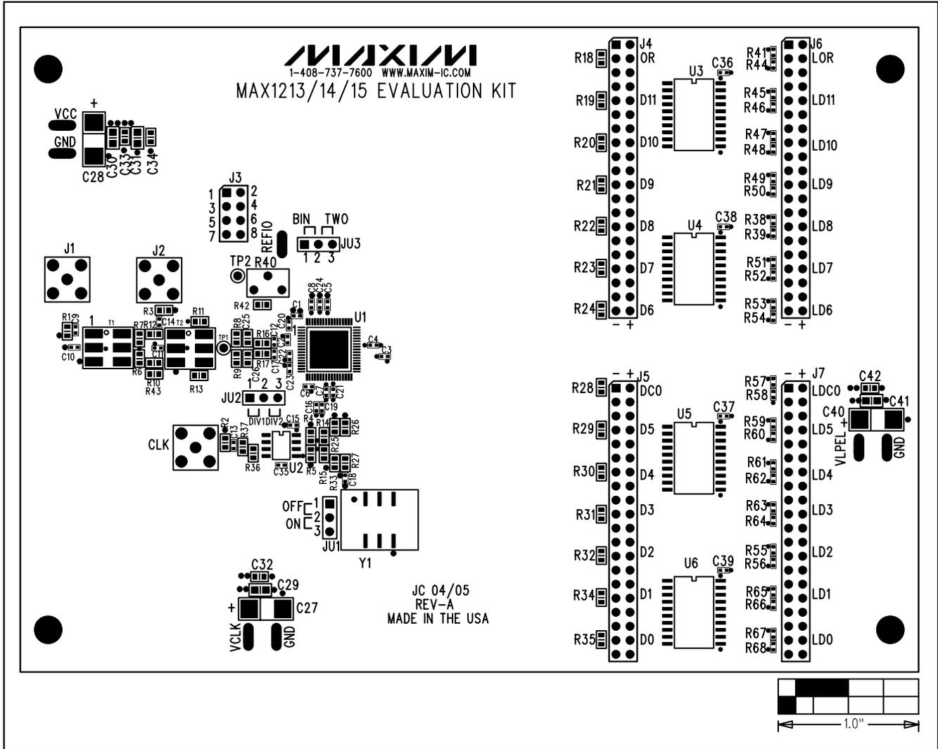
Figure 2. MAX1213/MAX1214/MAX1215 EV Kit Component Placement Guide—Component Side
