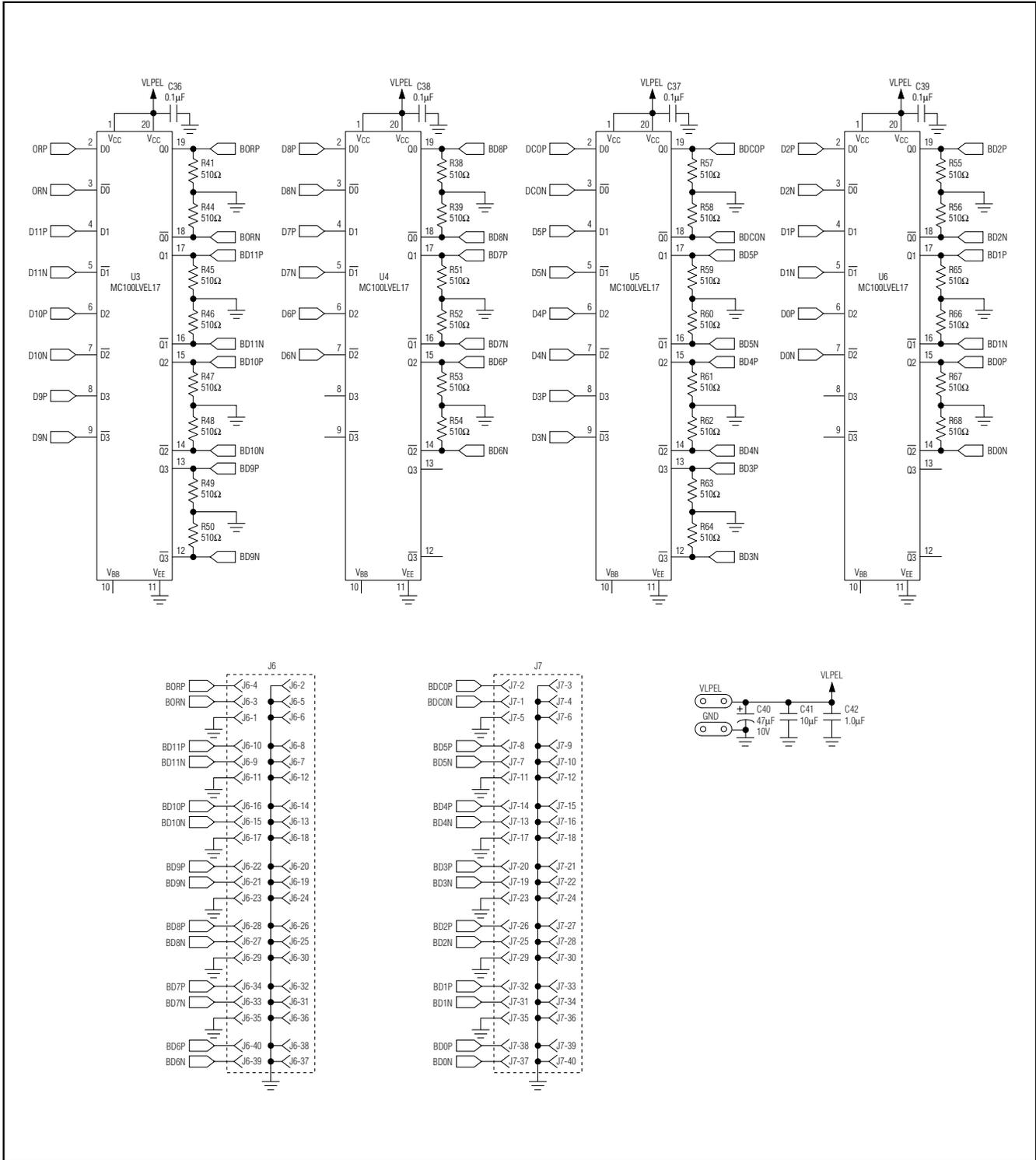
Figure 1. MAX1213/MAX1214/MAX1215 EV Kit Schematic (Sheet 2 of 2)
