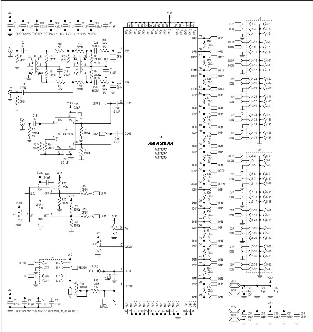
Figure 1. MAX1213/MAX1214/MAX1215 EV Kit Schematic (Sheet 1 of 2)
