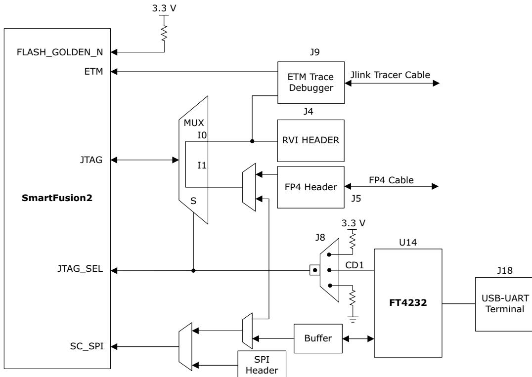
**JTAG\_SEL:** JTAG\_SEL is used to switch between the FlashPro4 header (high) and the RVI header or ETM header (low). For more information about the J8 jumper, see [Table 3](#), page 6.
