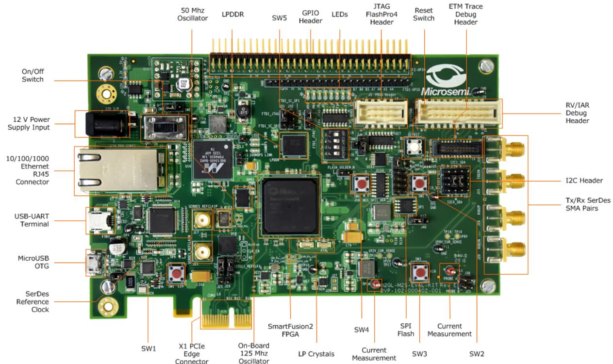
**Note:** Microsemi recommends using a 12-inch SMA Male to SMA Male Precision Cable using the RoHS-compliant PE-SR405FLJ coax with the SmartFusion2 Security Evaluation Kit. For more information, see [www.pasternack.com/sma-male-sma-male-pe-sr405flj-cable-assembly-pe39429-12-p.aspx](http://www.pasternack.com/sma-male-sma-male-pe-sr405flj-cable-assembly-pe39429-12-p.aspx).
