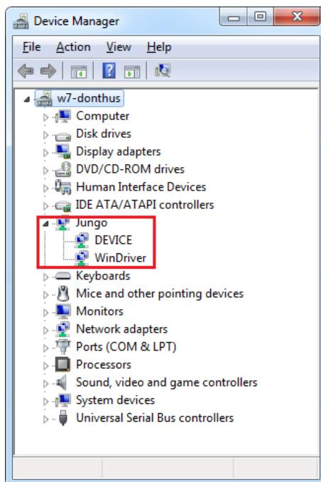
**Note:** If a warning symbol is displayed on the **DEVICE** or **WinDriver** icons in the Device Manager, uninstall and reinstall the drivers (see [Installing Drivers](#), page 58).
