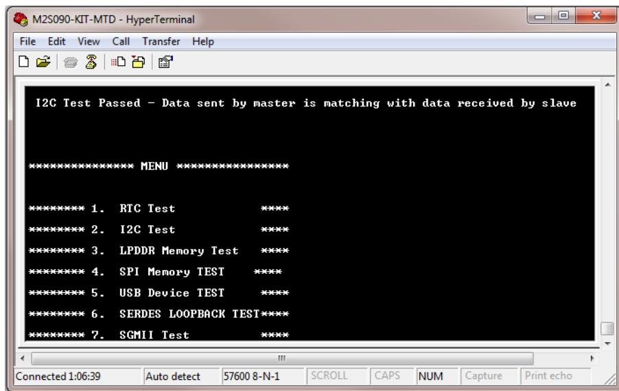
4. Press **3** to run the LPDDR memory test.
