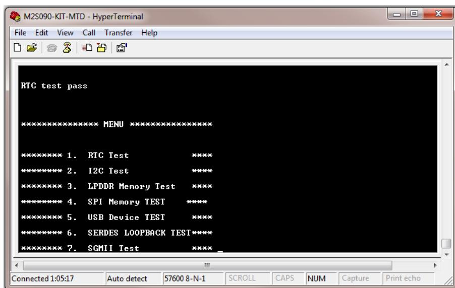
3. Press 2 to run the I2C loopback test.
