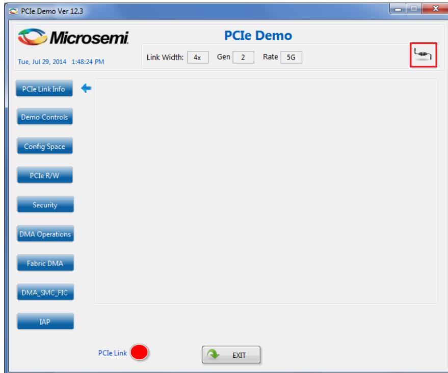
4. Click the **Connect** icon (highlighted in the above figure) at the top-right corner of the GUI. The link width, device generation (Gen 1/Gen 2), data rate, and kit type are displayed on the GUI, as shown in the following figure.
