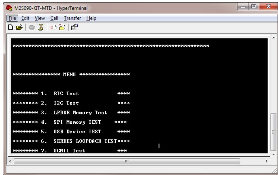
If the list of tests does not appear, press the **SW6** reset switch again. If the list still does not appear, then check all the jumpers, and the HyperTerminal settings.
