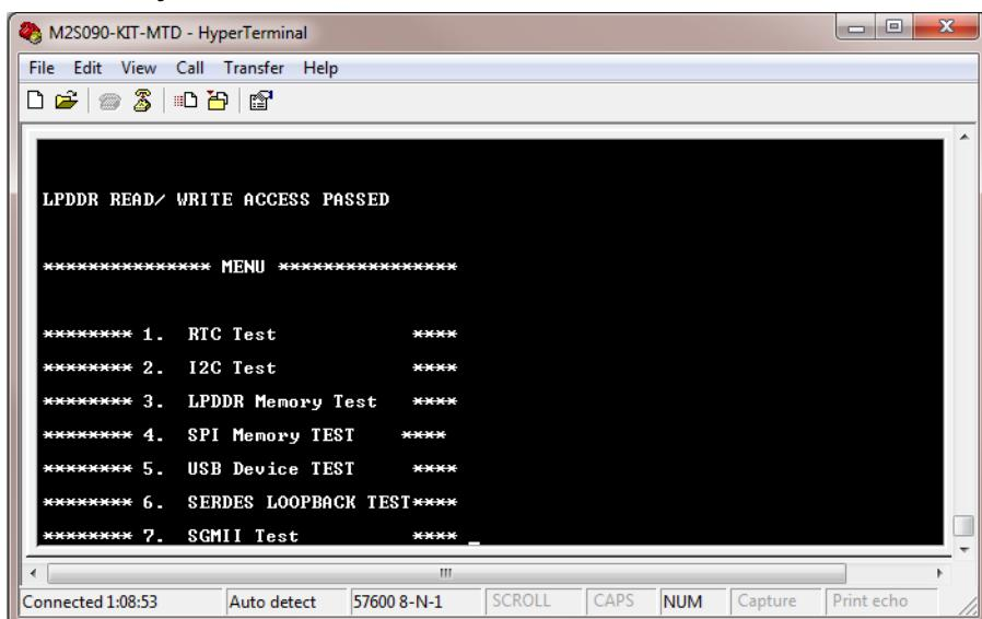
5. Press **4** to run the SPI memory test.
