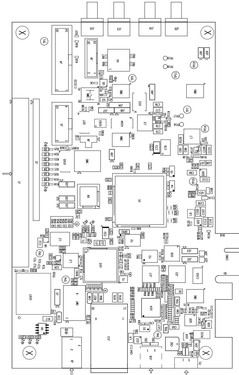
The following figure shows the bottom view of the SmartFusion2 Security Evaluation Kit silkscreen.
