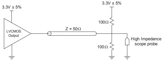
**Figure 2: XR81101 3.3V LVC MOS Output Termination**
