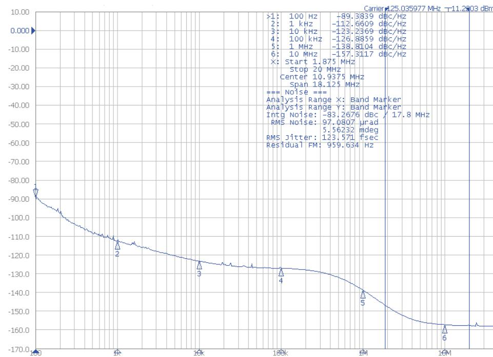
Figure 1: 125MHz Operation, Typical Phase Noise at 3.3V
