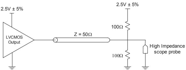
**Figure 3: XR81101 2.5V LVC MOS Output Termination**
