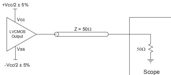
**Figure 4: XR81101 Split Supply LVC MOS Output Termination**
