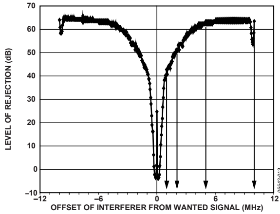
Figure 13. Wideband Interference Rejection; Wanted Signal (901 MHz, 38.4 kbps Data Rate, 200 kHz Frequency Deviation) at 6 dB Above Sensitivity Point; Interferer = CW Jammer
