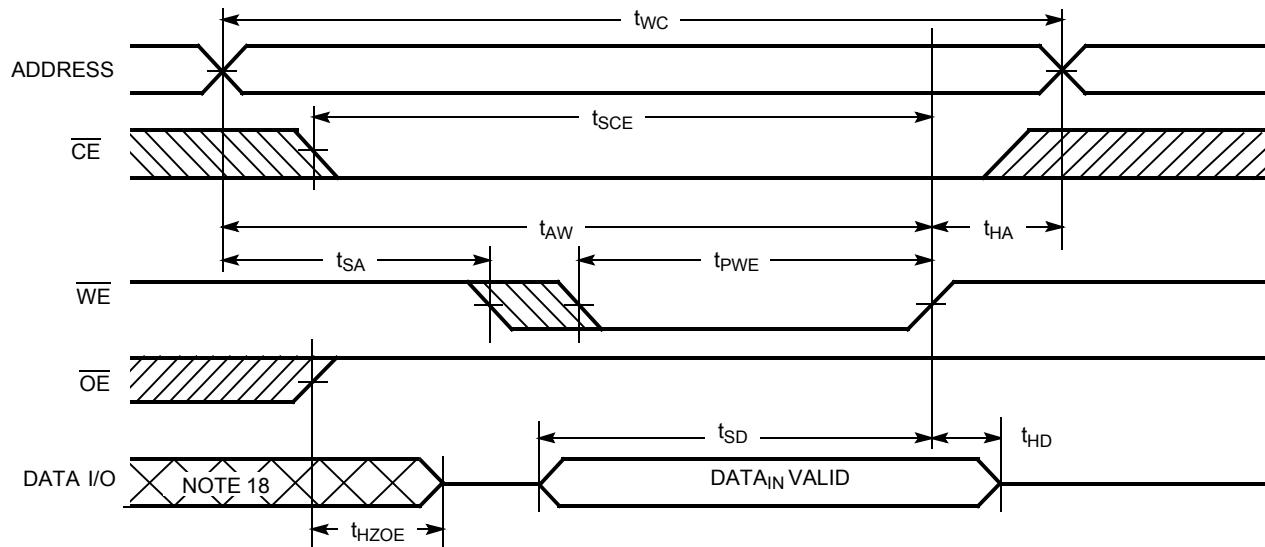
Figure 7. Write Cycle No. 3 ( $\overline{\text{WE}}$  Controlled,  $\overline{\text{OE}}$  LOW)
