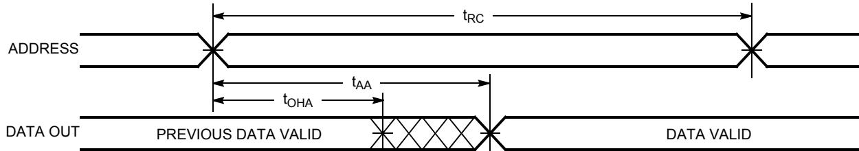
**Figure 4. Read Cycle No. 2 ( $\overline{OE}$  Controlled)** [12, 13]
