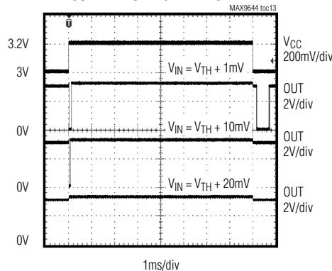
**POWER-SUPPLY REJECTION FOR NO FALSE TRIGGERING**
