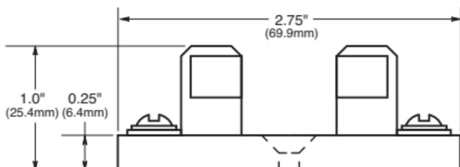
Note: Mounting screw hole diameter is 0.148" (3.7mm). Countersink, 0.313" (7.9mm). Max. mounting screw No. 6.
