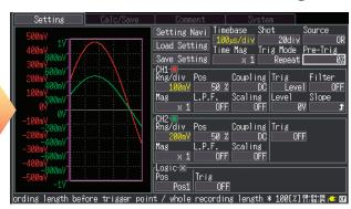
The help text crawls along the bottom of the screen, describing the function of the setting at the blinking cursor.
