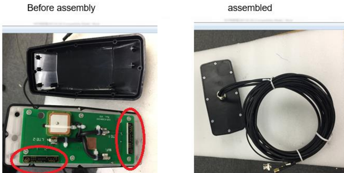
Fig.1: Appearance photos of the samples before test.
