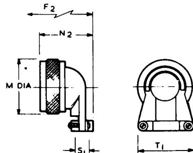
With Straight Strain Relief Saddle Clamp.
