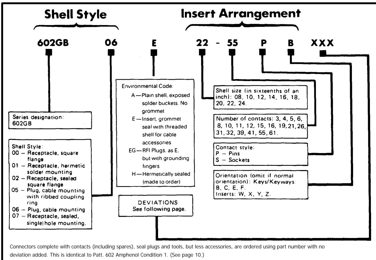
Connectors complete with contacts (including spares), seal plugs and tools, but less accessories, are ordered using part number with no deviation added. This is identical to Patt. 602 Amphenol Condition 1. (See page 10.)
