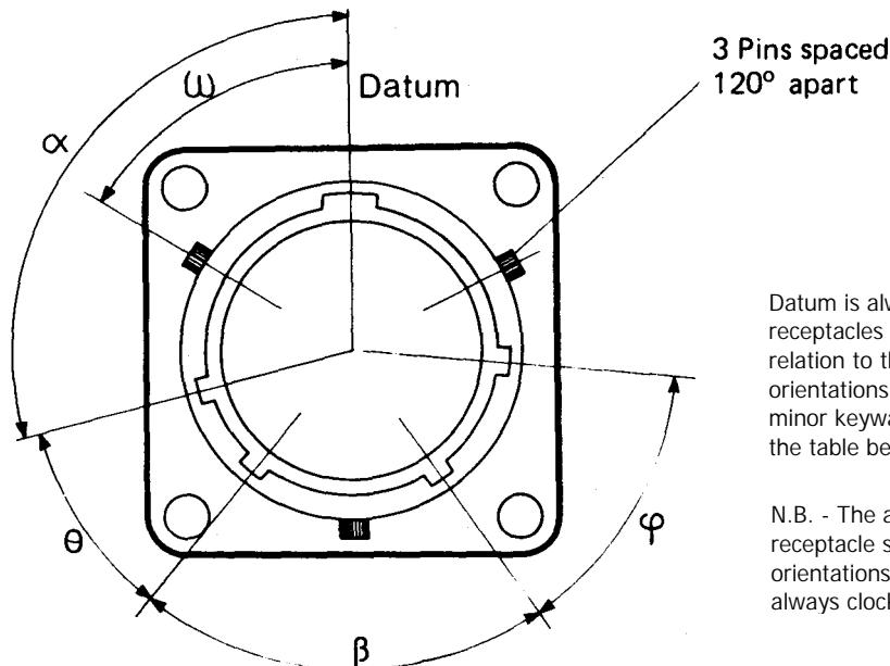
Datum is always taken from major key or keyway. In receptacles the major keyway always remains fixed in relation to the mounting flange. For the B,C,E and F orientations, the three bayonet locations and associated minor keyways are rotated complete, in accordance with the table below.
