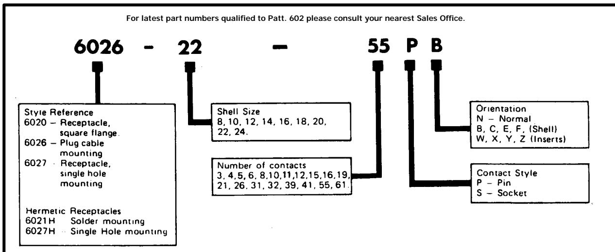
Connectors ordered against Patt. 602 numbers (as above) will be supplied in compliance with EL 2112 Patt. 602 requirements, this is a basic connector with the exact complement of contacts which comply with EL2113.
