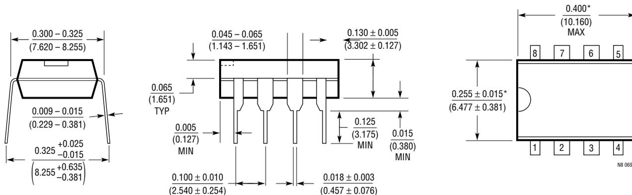
\*THESE DIMENSIONS DO NOT INCLUDE MOLD FLASH OR PROTRUSIONS.
