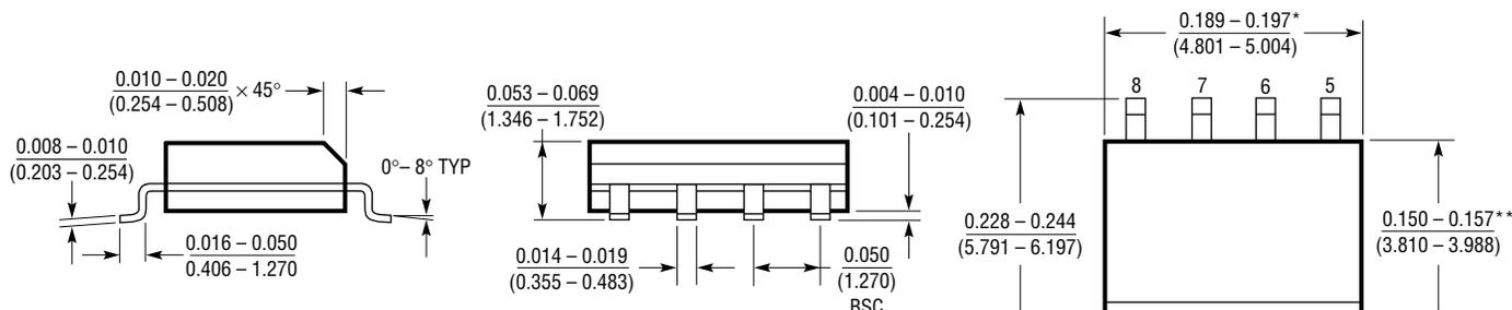
\*DIMENSION DOES NOT INCLUDE MOLD FLASH. MOLD FLASH SHALL NOT EXCEED 0.006" (0.152mm) PER SIDE
