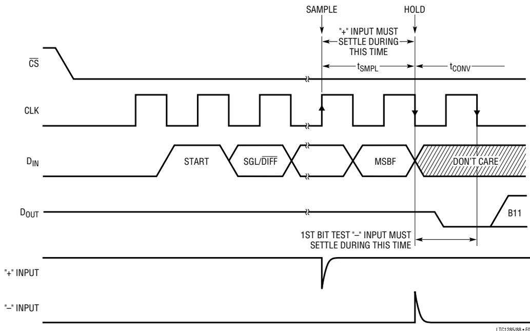
Figure 7. LTC1288 “+” and “-” Input Settling Windows
