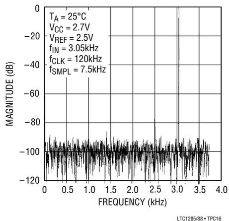
Figure 11. LTC1285 Non-Averaged, 4096 Point FFT Plot
