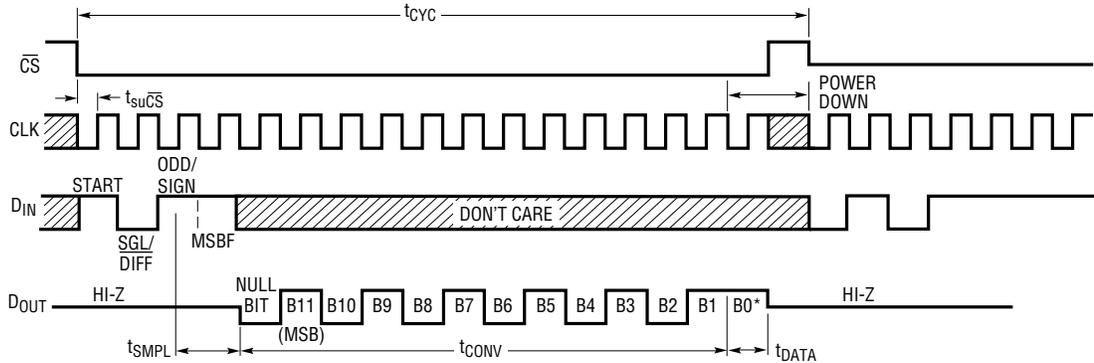
\*AFTER COMPLETING THE DATA TRANSFER, IF FURTHER CLOCKS ARE APPLIED WITH  $\overline{CS}$  LOW, THE ADC WILL OUTPUT ZEROS INDEFINITELY.
