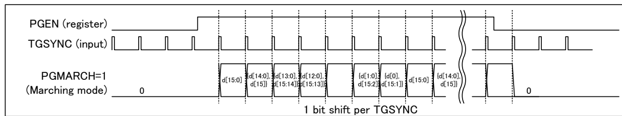
Figure 34 Test Pattern Output Data Formats (Marching mode)
