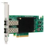
The Emulex OCe11102-I is a single-chip, high-performance 10Gb Ethernet (10GbE) adapter that consolidates traffic for networking and iSCSI storage. A member of the Emulex OneConnect Universal Converged Network Adapter (UCNA) family, the OCe11102-I iSCSI adapter supports CPU offload for both network and storage I/O to optimize server performance and maximize server virtualization ratios.
