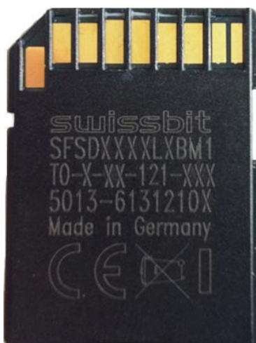
Example of the back side laser marking
