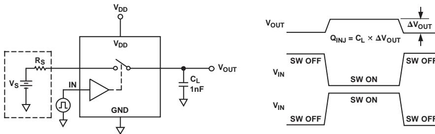
Figure 21. Charge Injection
