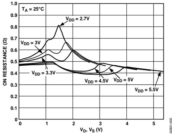
Figure 5. On Resistance vs.  $V_D$ ,  $V_S$
