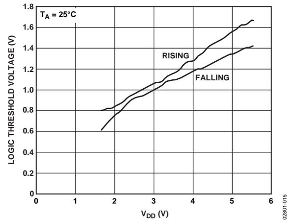
Figure 15. Logic Threshold Voltage vs. Supply Voltage
