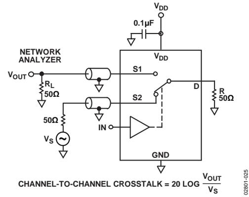
Figure 24. Channel-to-Channel Crosstalk
