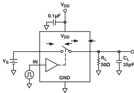
Figure 19. Switching Times
