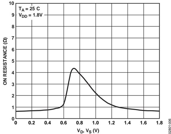
Figure 6. On Resistance vs.  $V_D$ ,  $V_S$
