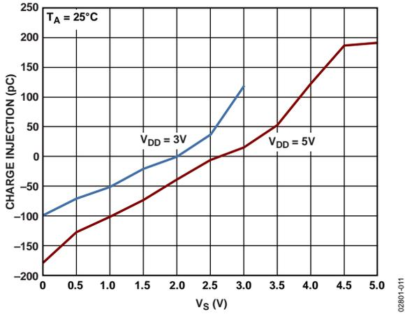
Figure 11. Charge Injection vs.  $V_S$  (Source Voltage)
