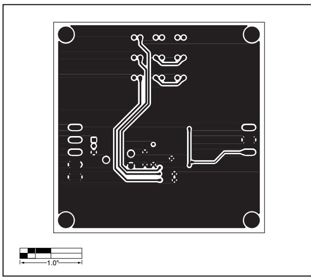
Figure 4. MAX1698 EV Kit PC Board Layout—Solder Side
