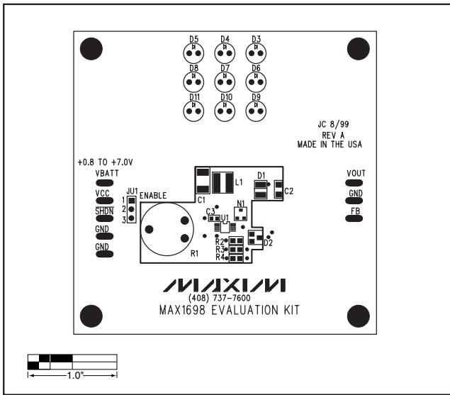
Figure 2. MAX1698 EV Kit Component Placement Guide—Component Side
