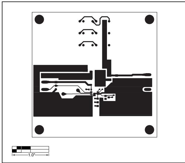
Figure 3. MAX1698 EV Kit PC Board Layout—Component Side
