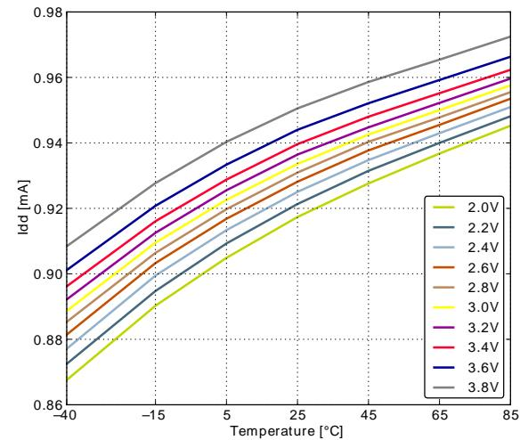
**Figure 3.5. EM1 Current consumption with all peripheral clocks disabled and HFRCO running at 11MHz**
