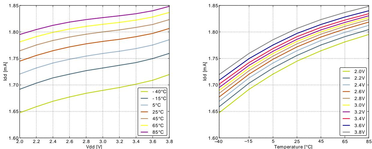
**Figure 3.3. EM1 Current consumption with all peripheral clocks disabled and HFRCO running at 21MHz**
