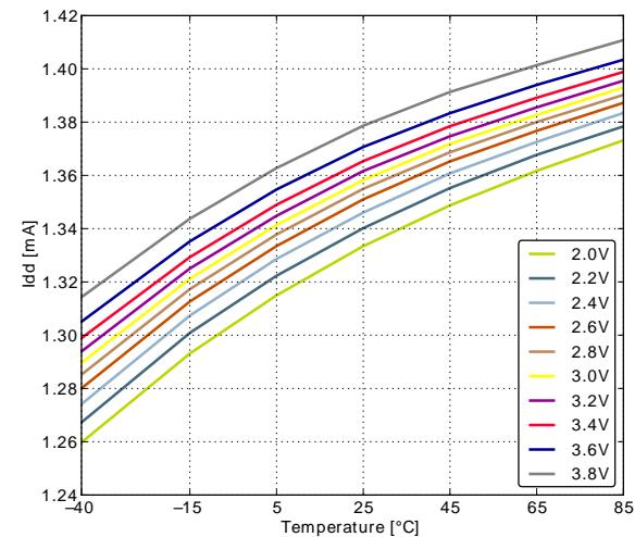
**Figure 3.4. EM1 Current consumption with all peripheral clocks disabled and HFRCO running at 14MHz**
