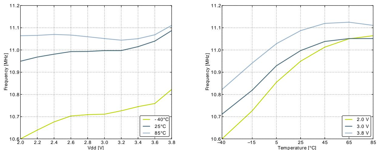
**Figure 3.21. Calibrated HFRCO 14 MHz Band Frequency vs Supply Voltage and Temperature**
