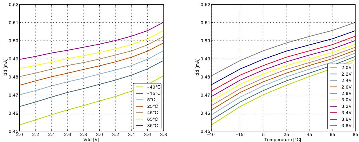
**Figure 3.7. EM1 Current consumption with all peripheral clocks disabled and HFRCO running at 1.2MHz**
