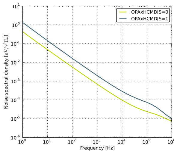
**Figure 3.36. OPAMP Voltage Noise Spectral Density (Non-Unity Gain)**
