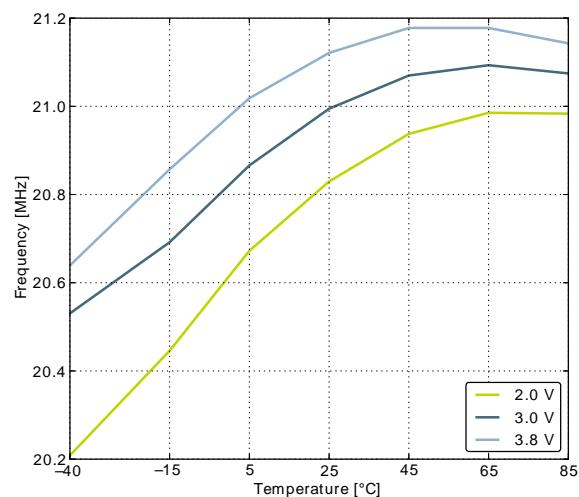
**Figure 3.23. Calibrated HFRCO 28 MHz Band Frequency vs Supply Voltage and Temperature**
