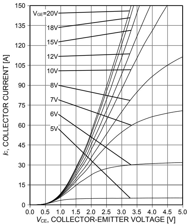
**Figure 5. Typical output characteristic**
