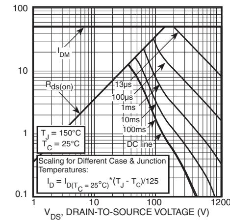
**Figure 10, Maximum Forward Safe Operating Area**
