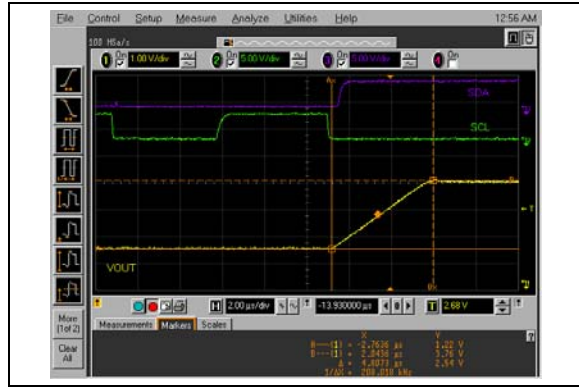
FIGURE 2-98: Half-Scale Settling Time (400h to C00h) (MCP4726).
