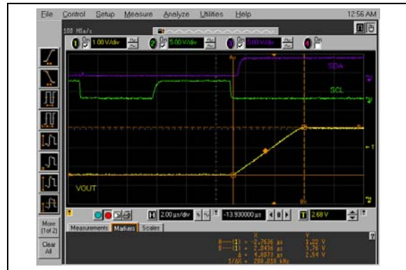
FIGURE 2-98: Half-Scale Settling Time (400h to C00h) (MCP4726).
