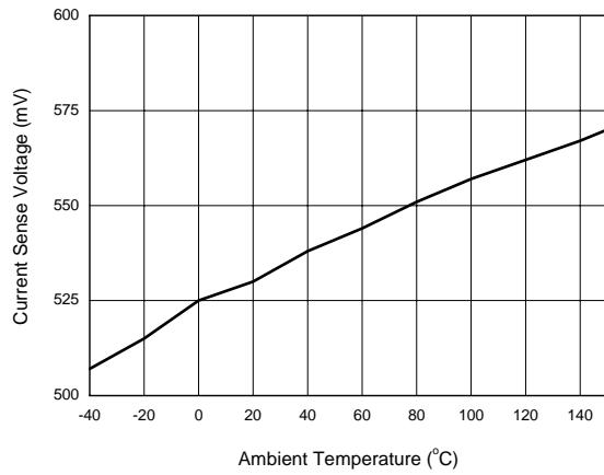
Figure 12. Current Sense Voltage
