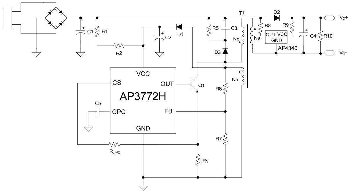
Figure 18. 5V/1A Output for Battery Charger of Mobile Phone
