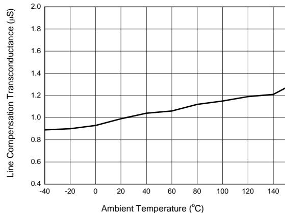
Figure 17. Line Compensation Transconductance vs. Ambient Temperature
