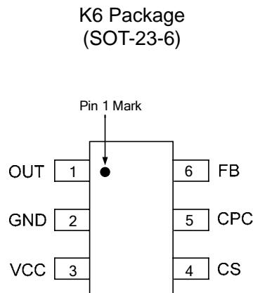
Figure 2. Pin Configuration of AP3772H (Top View)
