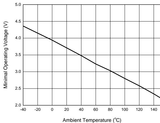
Figure 6. Minimal Operating Voltage vs. Ambient Temperature
