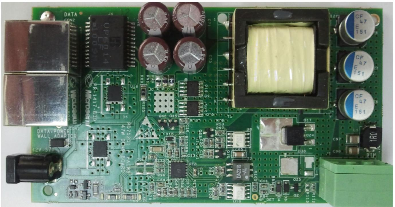
**Figure 2: PD70201EVB47F Evaluation Board – General View**
