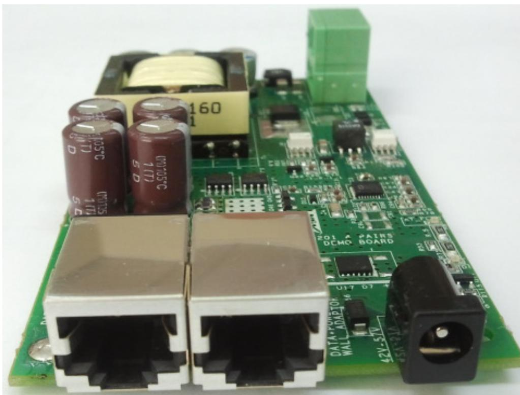
Figure 3: Front RJ45 and Wall Adapter Connectors
