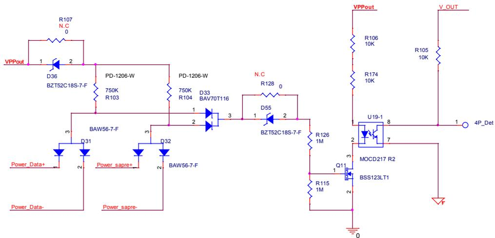
Figure 6: 4P\_DET indication Circuit
