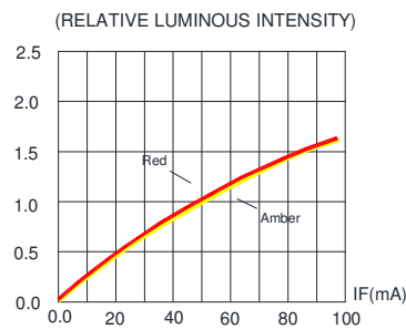
FIG.2 RELATIVE LUMINOUS INTENSITY VS. FORWARD CURRENT
