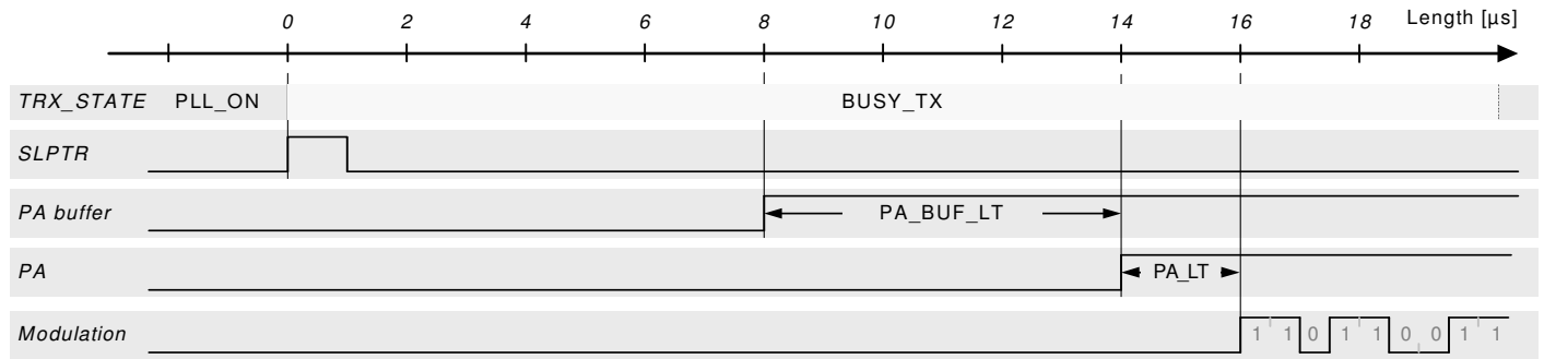
Figure 9-22. TX Power Ramping
