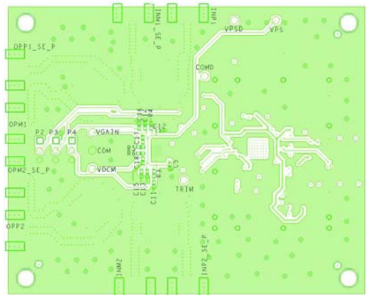
Figure 61. Component Side Layout
