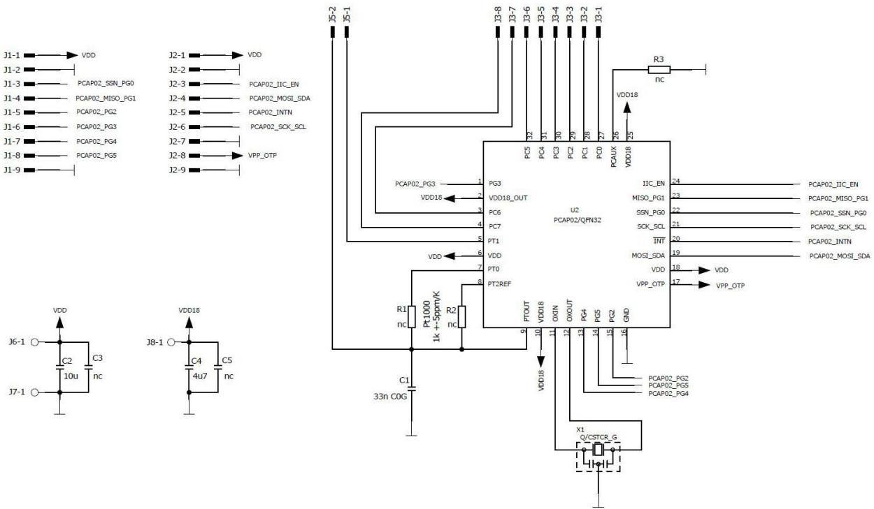
Figure 4-2: PCaO2 AD module schematics
