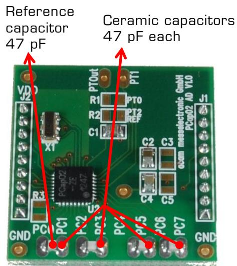
Figure 2-2: Details of the plug-in module
