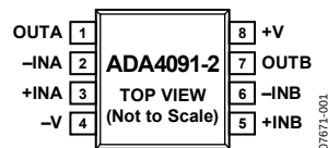
Figure 1. 8-Lead, Narrow-Body SOIC (R-8)
