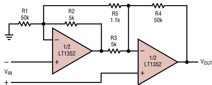
$$\text{GAIN} = [R_4/R_3][1 + (1/2)(R_2/R_1 + R_3/R_4) + (R_2 + R_3)/R_5] = 102$$
