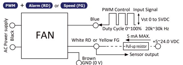
Note: Standard Qualtek EC fans have either 2 lead wires, or terminals
